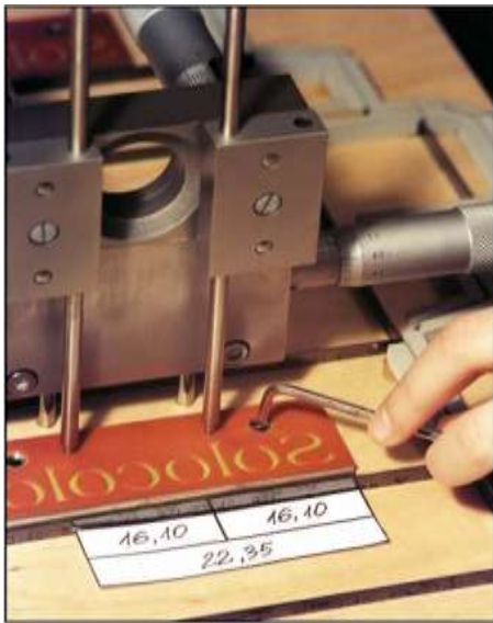
Fig. 3 The example of holes positioning in the die board and matrix.
